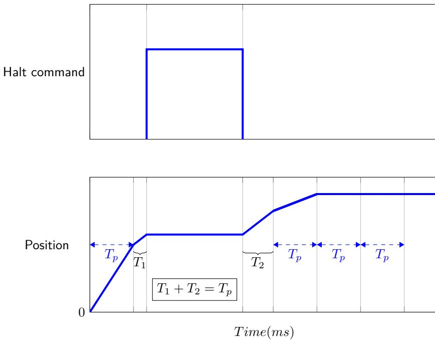
Figure 1.95: Halt Command Operation Graph
