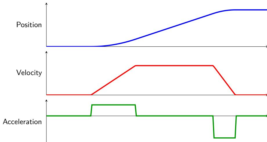
Figure 1.69: Linear ramp (trapezoidal profile)
