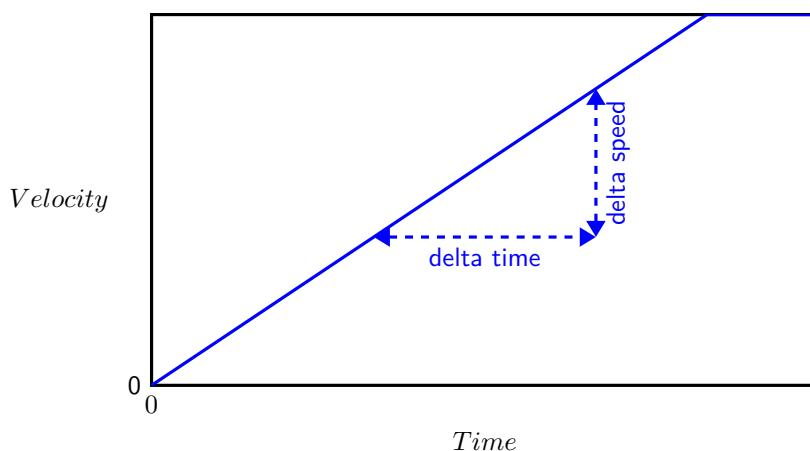
Figure 1.51: Feature of acceleration ramp
