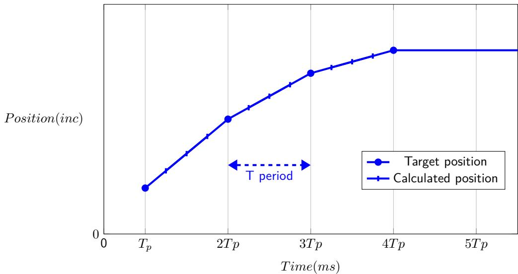
Figure 1.94: Linear interpolation
