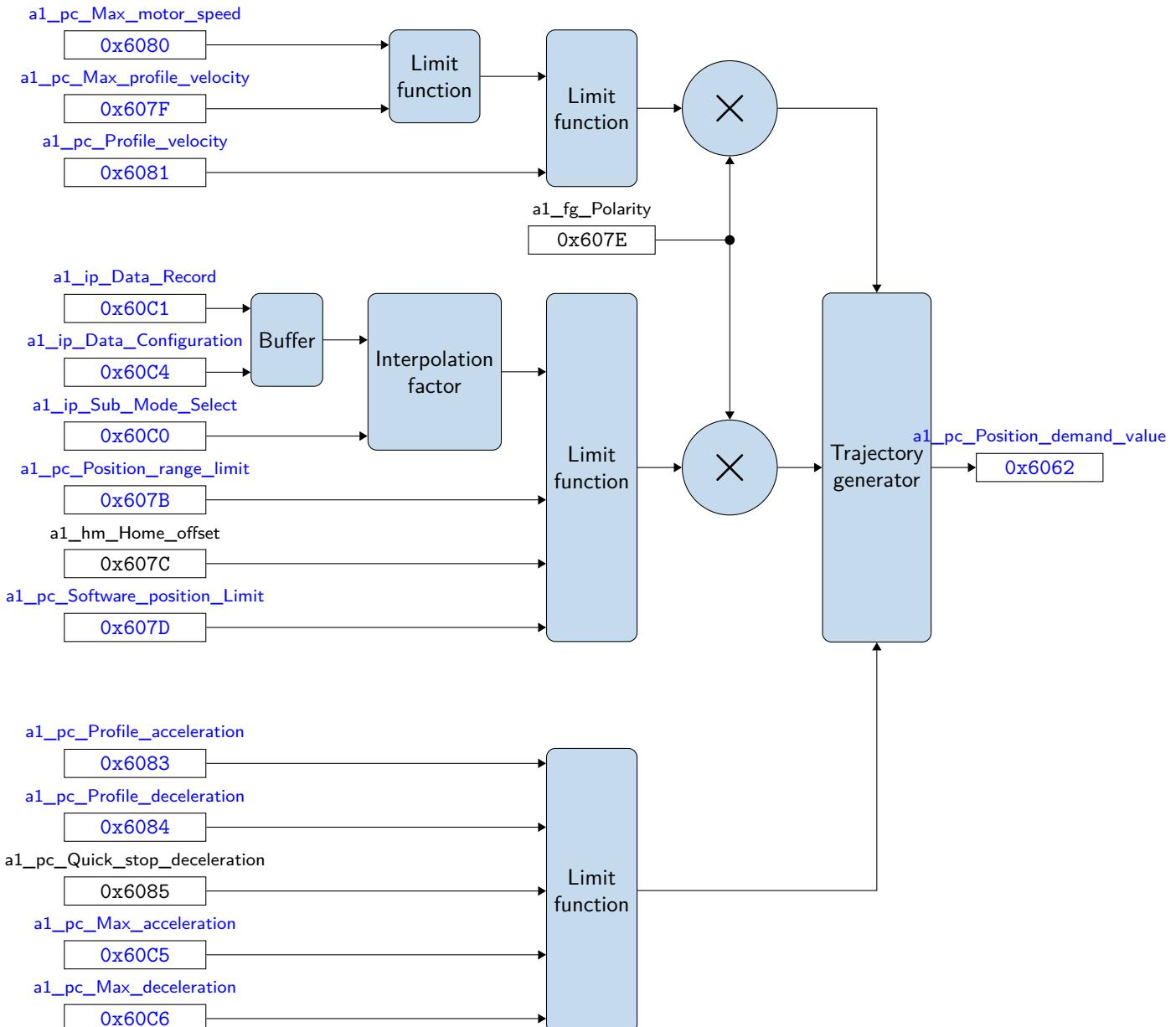
Figure 1.91: functional diagram of Interpolated position mode with all objects
