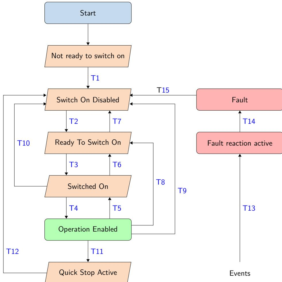
Figure 1.1: State machine of 402
