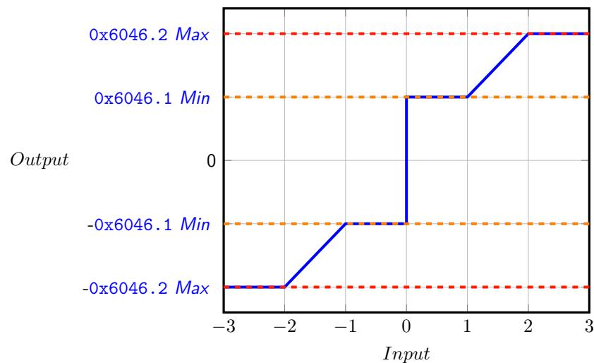
Figure 1.47: Characteristic of minimum and maximum of velocity
