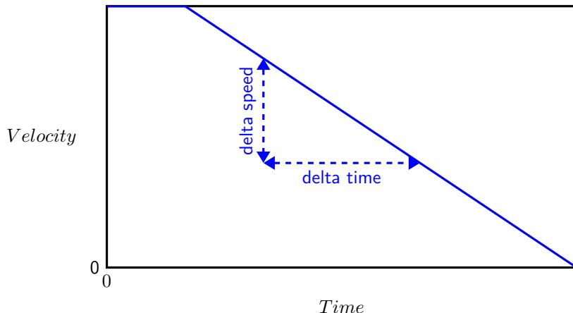
Figure 1.54: Feature of deceleration ramp
