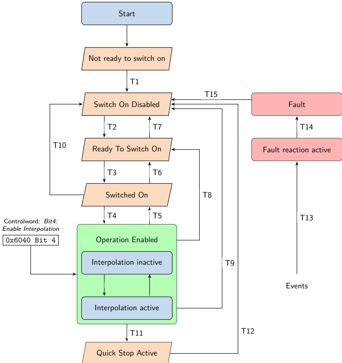
Figure 1.92: State machine of Interpolated position mode
