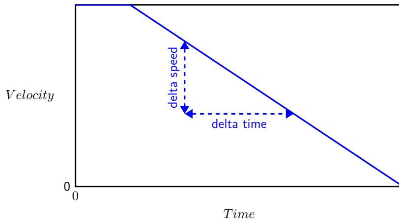
Figure 1.57: Feature of deceleration ramp for quick stop
