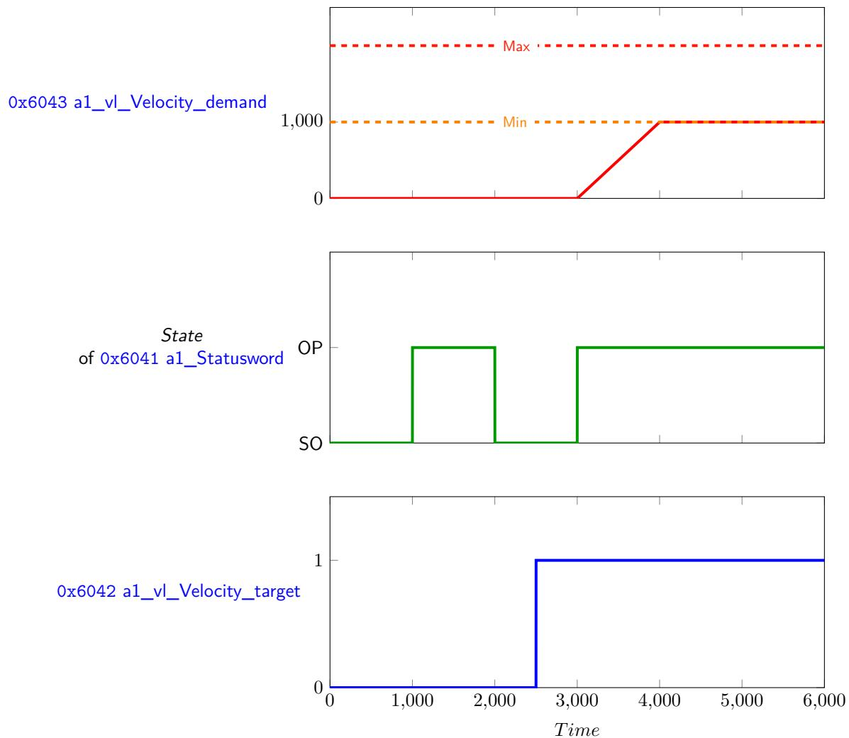
Figure 1.48: Special case when going from "Switched On(SO)" state to "Operation Enabled(OP)" state
