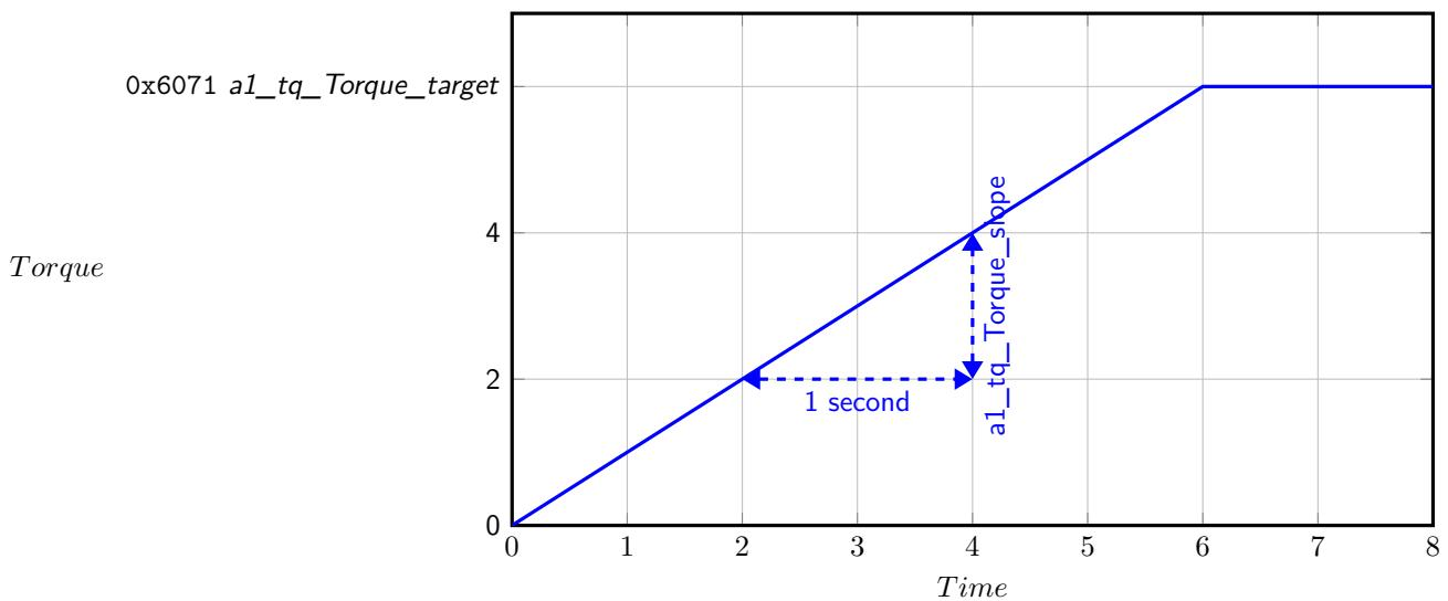
Figure 1.25: Feature of torque ramp
