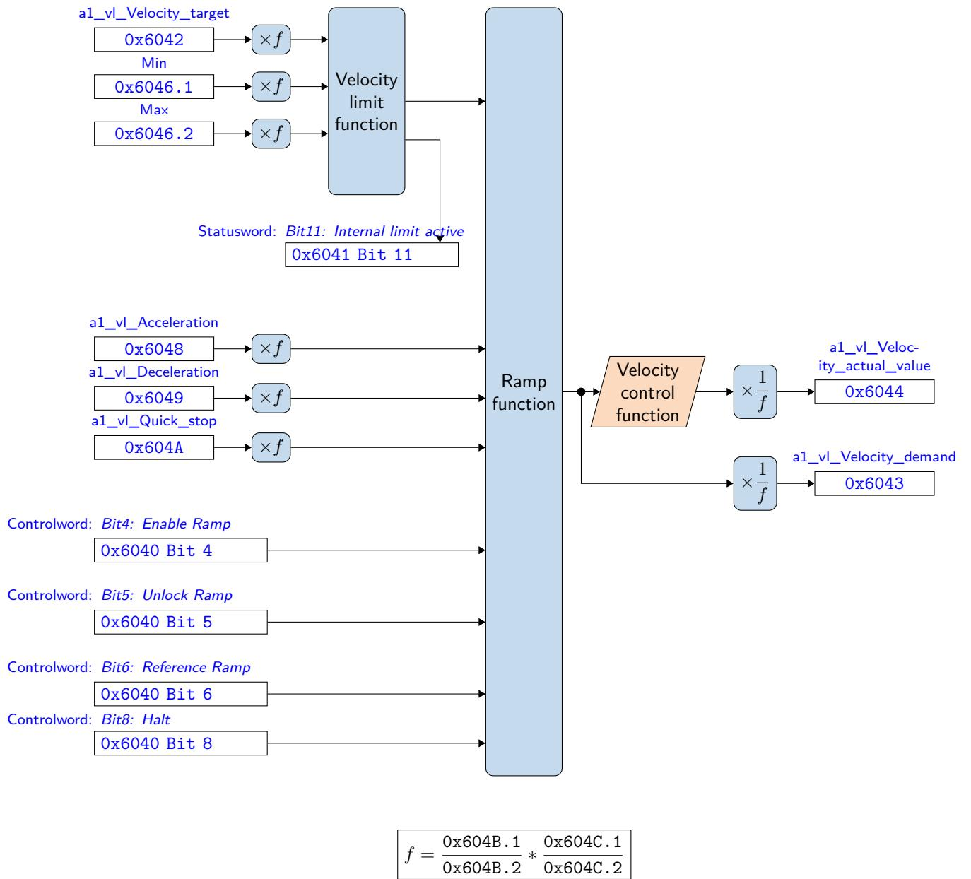
Figure 1.35: functional diagram of Velocity mode with all objects
