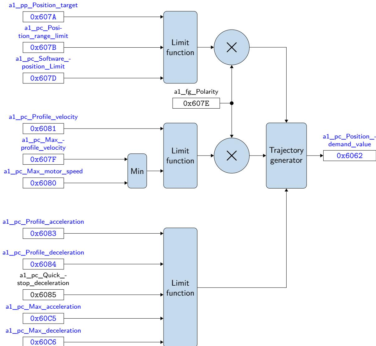
Figure 1.66: functional diagram of Profile Position Modewith all objects
