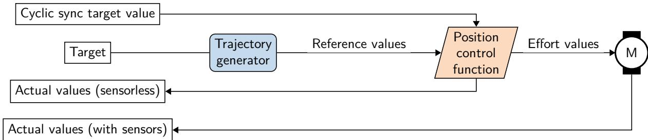
Figure 1.90: Interpolated position mode
