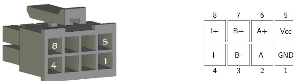
Figure 1.8: J301 pins, 2 x 4 pins, main sensor input
