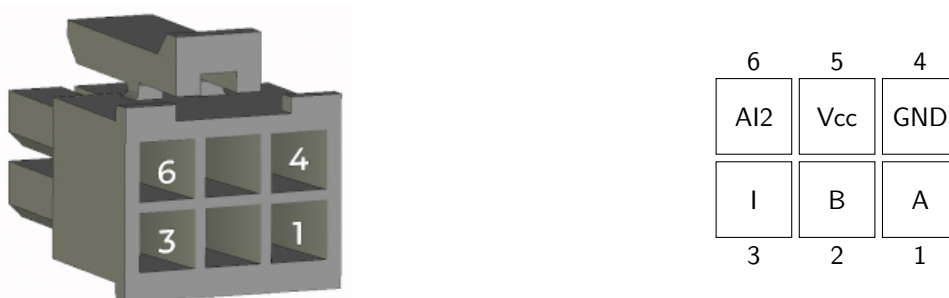
Figure 1.10: J401 pins, 2 x 3 pins, auxiliary sensor input
