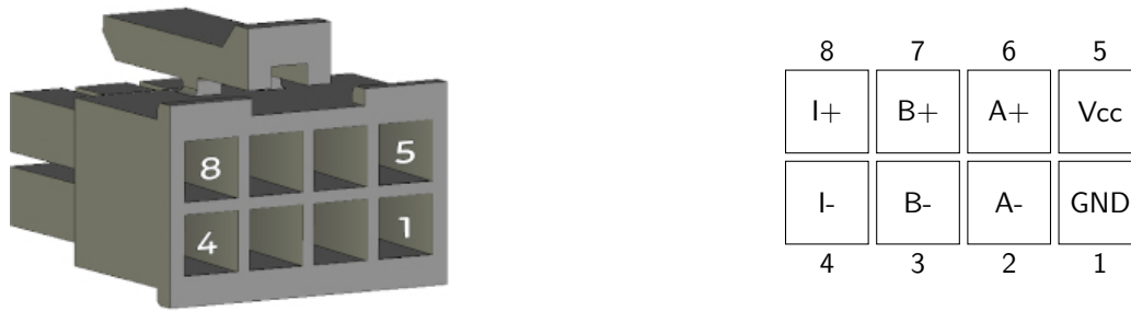
Figure 1.8: J301 pins, 2 x 4 pins, main sensor input
