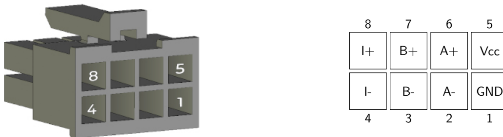
Figure 1.7: J301 pins, 2 x 4 pins, main sensor input
