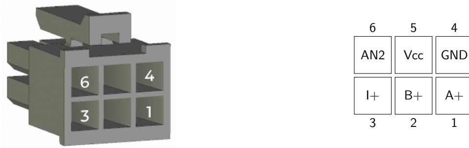
Figure 1.9: J401 pins, 2 x 3 pins, auxiliary sensor input
